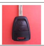
Next fit assembled key buttons and red plate in the top part of your remote. Once key buttons are in, you will place electronic component over the top part of the shell. Next you can cover it with bottom part of the hard shell. If all components sit in correctly you can close remote by firm pressing and screw to pieces together. Your refurbished remote should look like the one in the picture above. No re-programming is need it.
