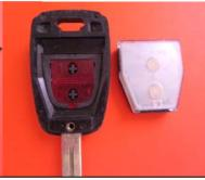
Unscrew small screw at the back of plastic shell. Praise open remote placing your fingernail in the small cut out located at the key shaft end. Separate all parts: top hard shell part with button key pad with electronic board and back part of the shell.
